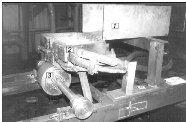
Figure 4. Technological fixture mounted on a moveable frame: 1 — non-consumable box; 2 — cold hearth; 3 — drum-type mould
