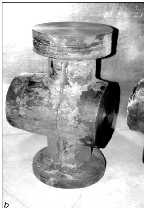
Figure 3. Scheme ( a ) and appearance ( b ) of billet of CT shaft valve with 80 mm diameter passing section produced by the method of electroslag casting (thin lines show the external contour of a ready component)
