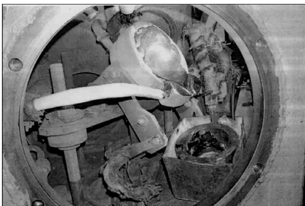
Figure 2. Melting chamber with a crucible and mould for a pressed billet remelting
