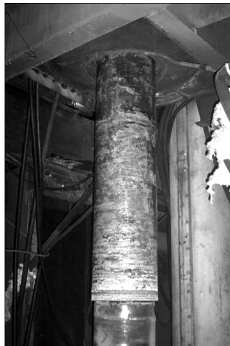
Figure 5. Bimetal ingot of 350 mm diameter after electroslag cladding of corrosion-resistant austenitic layer of 35 mm thickness using method of ESR LM
