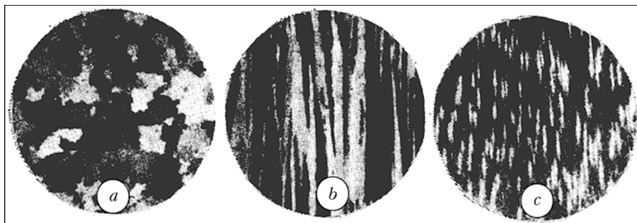
Figure 1. Macrostructure of heat-resistant alloys in GTE blades: a --- equiaxial; b --- directional columnar; c --- single-crystal ( \times 300 )
