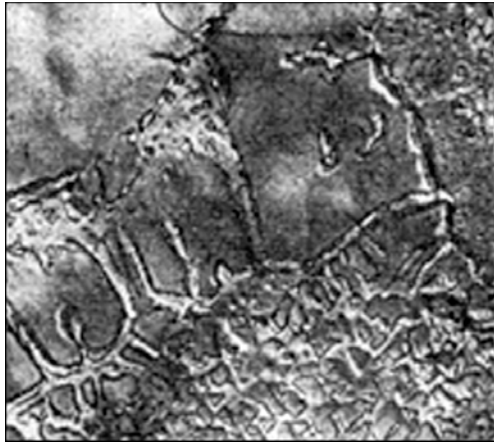
Figure 2. Microstructure of high-strength foundry heat-resistant alloy. Eutectics \gamma + \gamma' ( \times 8000 )
