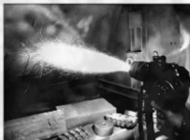
The system comprises electric arc metalliser, wire feed mechanism and power supply. The equipment is mobile and can operate both in manual and mechanised modes. Compared with traditional electric arc equipment, the system with the spraying unit of a new design provides increase in the velocity of a high-temperature jet, possibility of formation of contracted gas plume, increased density and low oxidation degree of coatings, as well as high strength of adhesion to the substrate:
