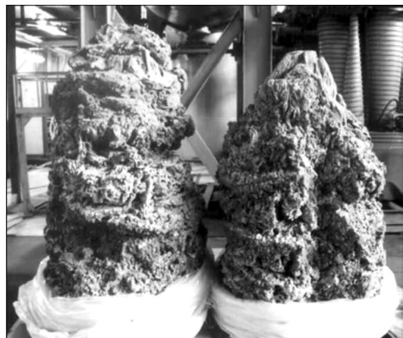
Figure 1. Appearance of spongy titanium blocks
