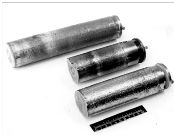
Figure 2. IMSM ingots melted from wastes of granulated powders of VT5-1kt alloy
