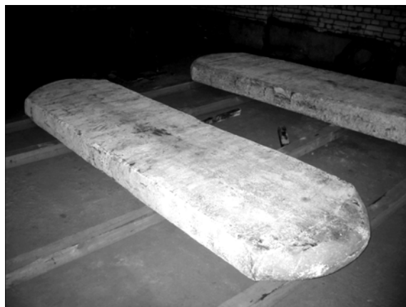
Figure 4. Malleated slabs of titanium of Grade 2
