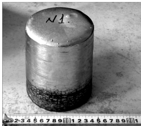
Figure 3. ESR ingot from TG-110 titanium sponge (melt 1)
