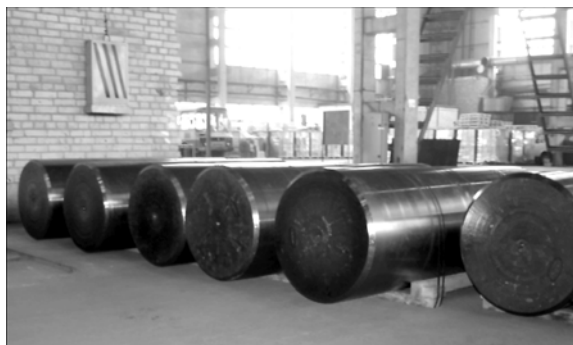
Figure 1. Ingots from titanium of Grade 2
