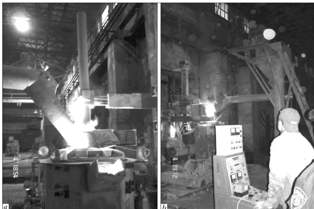
Figure 4. Melting of vanadium slag in electroslag furnace: a — furnace; b — melting process
