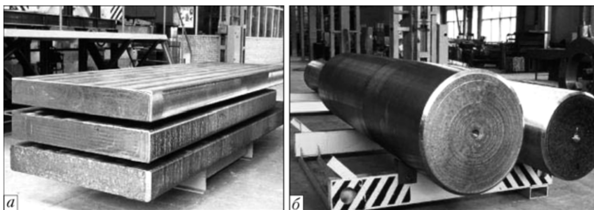
Fig. 11. External appearance of billets produced at the Antares company: a) rectangular cross-section 190 × 1325 mm; cylindrical billets diameter 825 mm.
