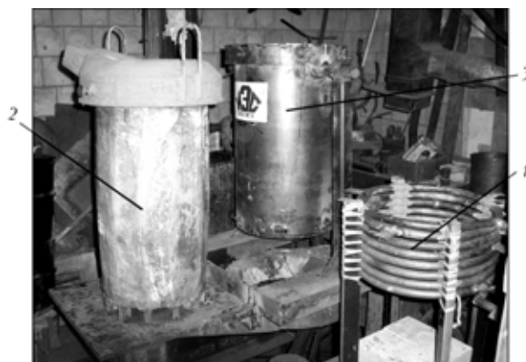
Fig. 2. General view of the melting-pouring module: 1) induction coil; 2) ladle; 3) pouring module.
