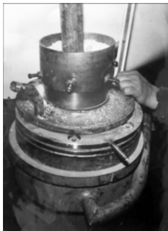
Fig. 3. A flux gate with a device for blowing with argon.
