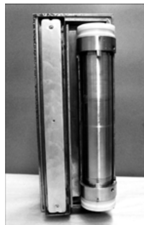
Fig. 8. General view of a cathode section for glow discharge and the arcotron with a cobalt cathode.
