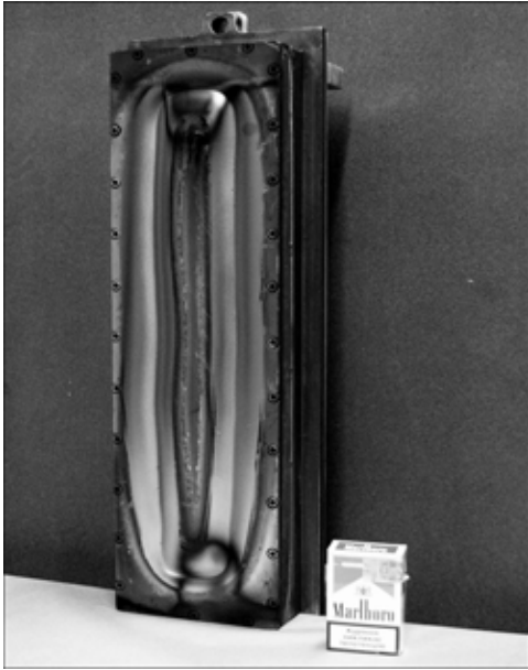
Fig. 5. General view of the modernised magnetron with direct cooling of the target-cathode.
