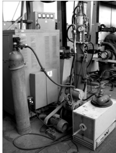
Fig. 2. General view of the chamber furnace for electroslag remelting with dosing devices and a power source.
