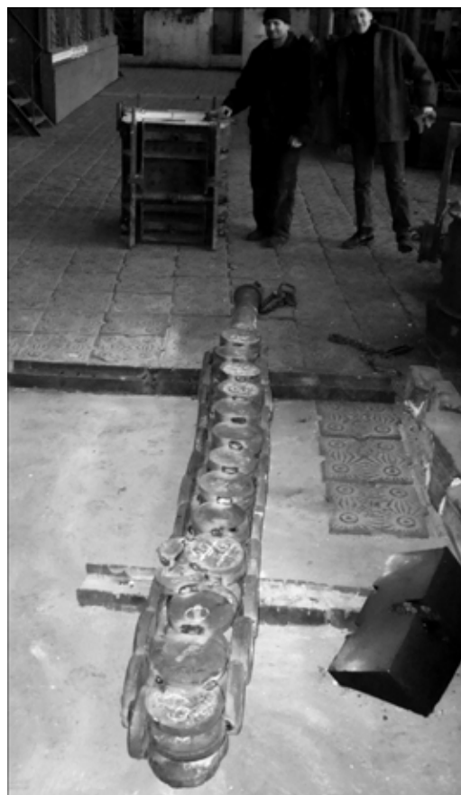
Fig. 1. A composite consumable electrode produced from the waste of KhN73MBTYu alloy.
