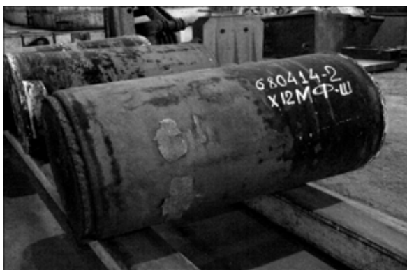
Fig. 6. ESR ingots with a diameter of 800 mm in Kh12MF-Sh steel, produced in ESR of the electrode with a cross-section of 370 \times 370 mm with increased supplied power.
