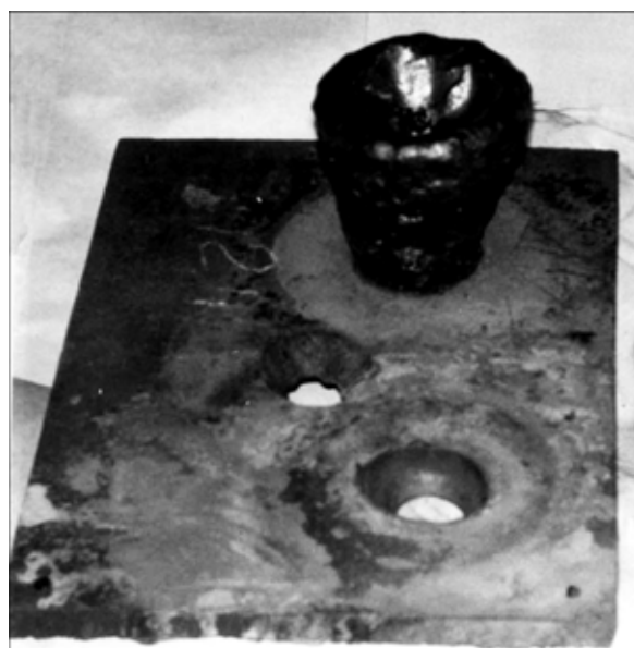
Fig. 5. A steel sheet 20 mm thick with holes melted by the jet of molten steel, with the blank for melting.
