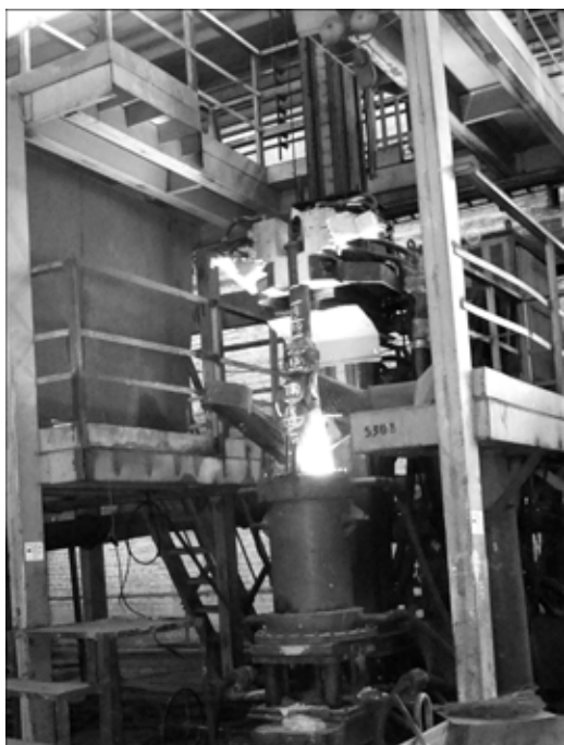
Fig. 2. Fragment of melting an ingot of KhN73MBTYu alloy in the USh-116 equipment.
