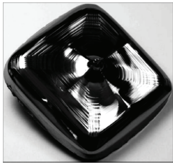
Fig. 4. Silicon single crystal, grown by the Czochralski method [12].
