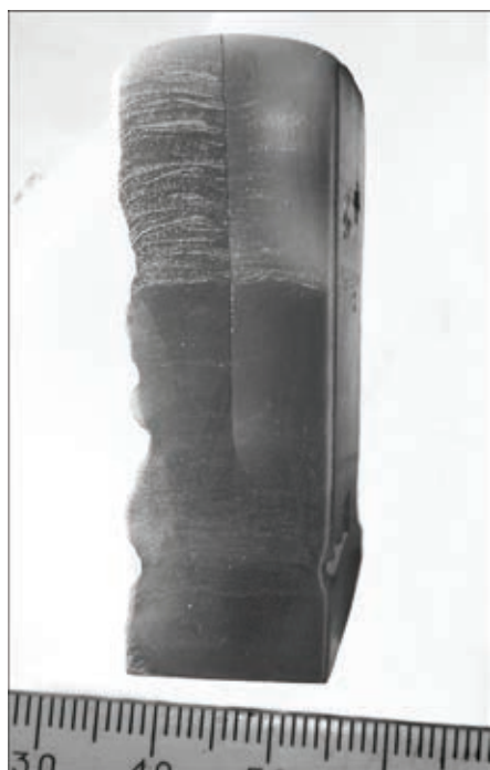
Fig. 4. Microstructure of the cross-section of a tungsten single crystal (110).
