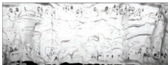
Fig. 1. Gas porosity at the melted end of a nickel ingot in the zone of contact with the walls of the solidification mould.
