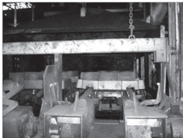
Fig. 5. Pallets with blanks stamped parts prior to boarding the heat wave.
