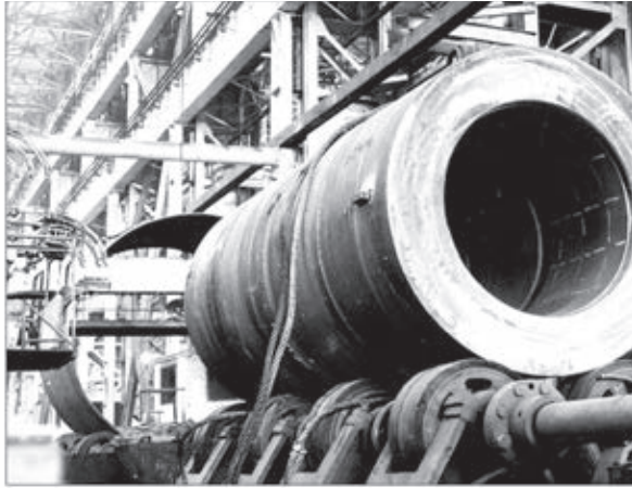
Fig. 11. Electroslag welding of the shipping container housing TK10 shells of thick-walled stainless steel with soldered lining.
