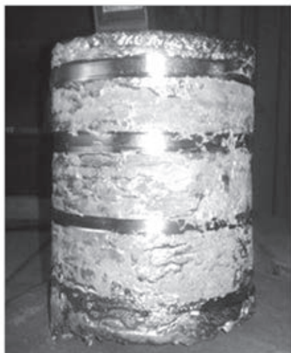
Fig. 2. Ingot of the TiAl intermetallic alloy after double remelting.
