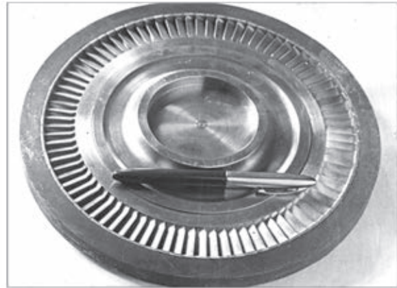
Fig. 2. Disk with blades assembled ring technology solder under pressure.
