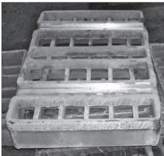
Fig. 4. View on trays after cleaning and machining.
