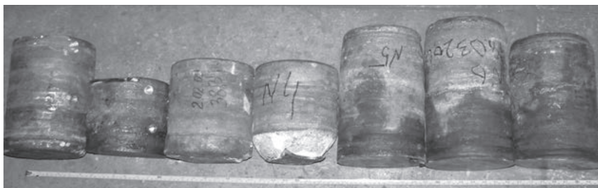
Fig. 4. External appearance of a pilot planned batch of billets of stainless steel melted from compacted electrodes.
