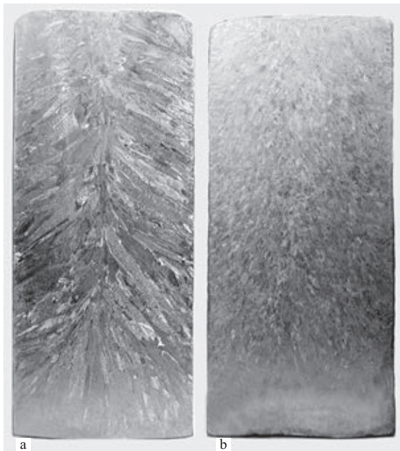
Fig. 16. Macrostructure of titanium ingots ESR, melted without electromagnetic effects (a) and with (b).
