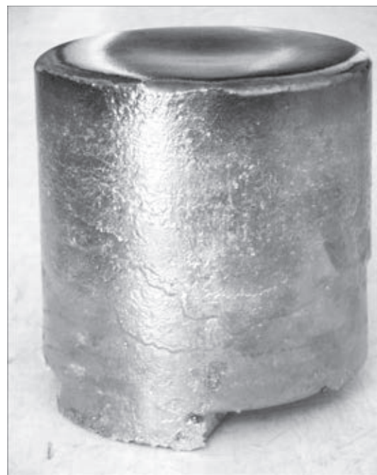
Fig 3. A billet of TiNi alloy.
