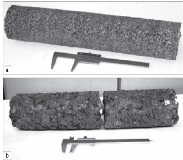
Fig. 4. Blank compacted from 100% fine steel shavings of SkKh15SG steel (a) and the large shavings of EP609-Sh creep resisting alloy (b).
