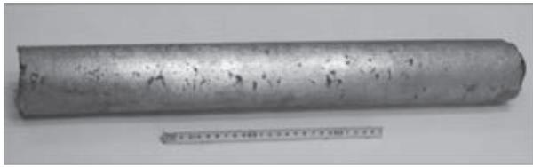
**Fig. 4.** The electrode with a diameter of 75 mm, compacted from titanium sponge.
