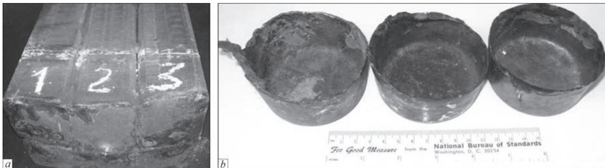
**Fig. 3.** External appearance of the consumable electrode (a packet of welded glass) with the melted end (a) and also sample of liquid metal of the ‘cup’ type in ESS LM (b).
