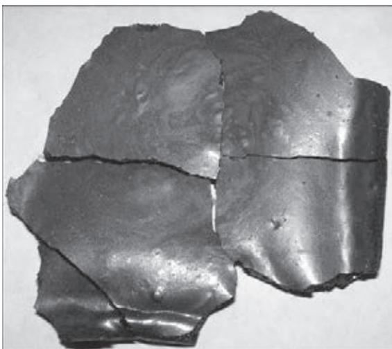
**Fig. 6.** Slag on the surface of the ingot.
