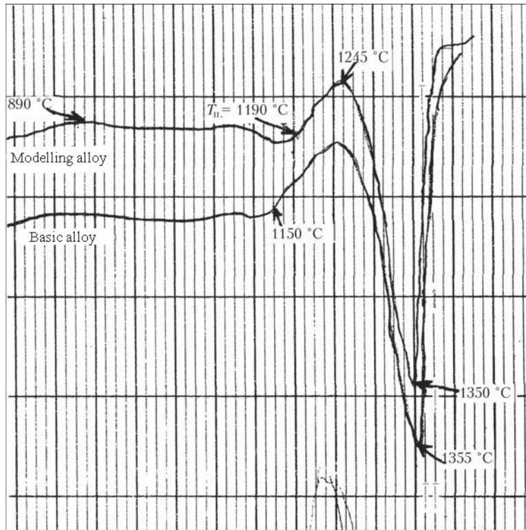
**Fig 1.** Values of the temperature of the main phase transformations ( $T_s$ ,  $T_L$ ,  $T_{c,d}$ ) of the simulation (1.5% rhenium and 1.5% tantalum) and basic alloys.
