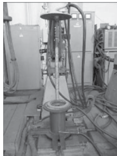
Fig. 5. The chamber electroslag furnace based on equipment A-550.
