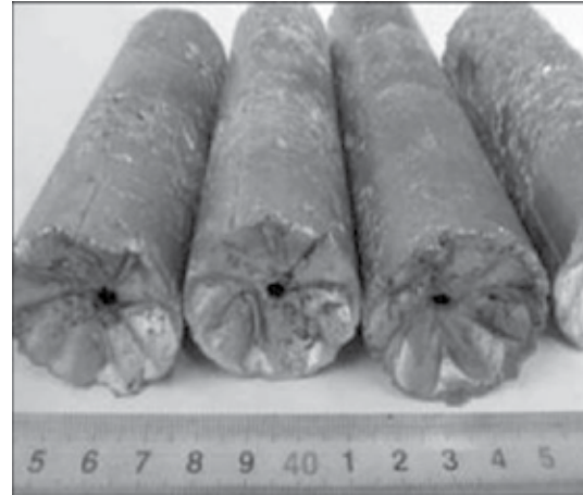
Fig. 4. Blocks of titanium sponge with the carbon powder pressed into the axial orifice.
