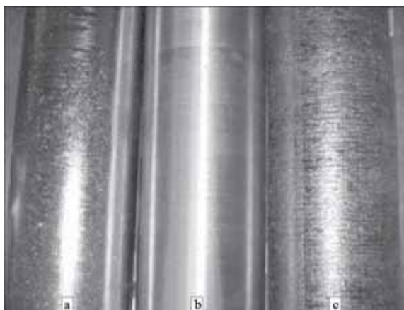
Fig. 7. External appearance of the surface of titanium alloy ingots: a) melted; b) machined; c) the cast ingot.
